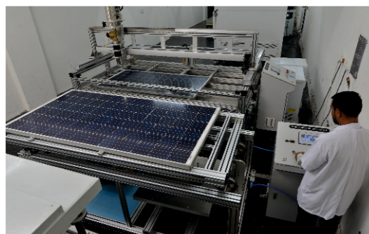
Robustness of Terminations Test Setup
