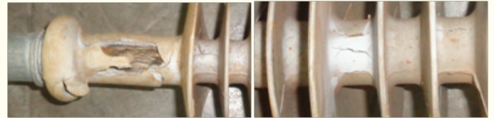
Figure 2.2.2(a): Images of damaged sections of silicone rubber insulator
