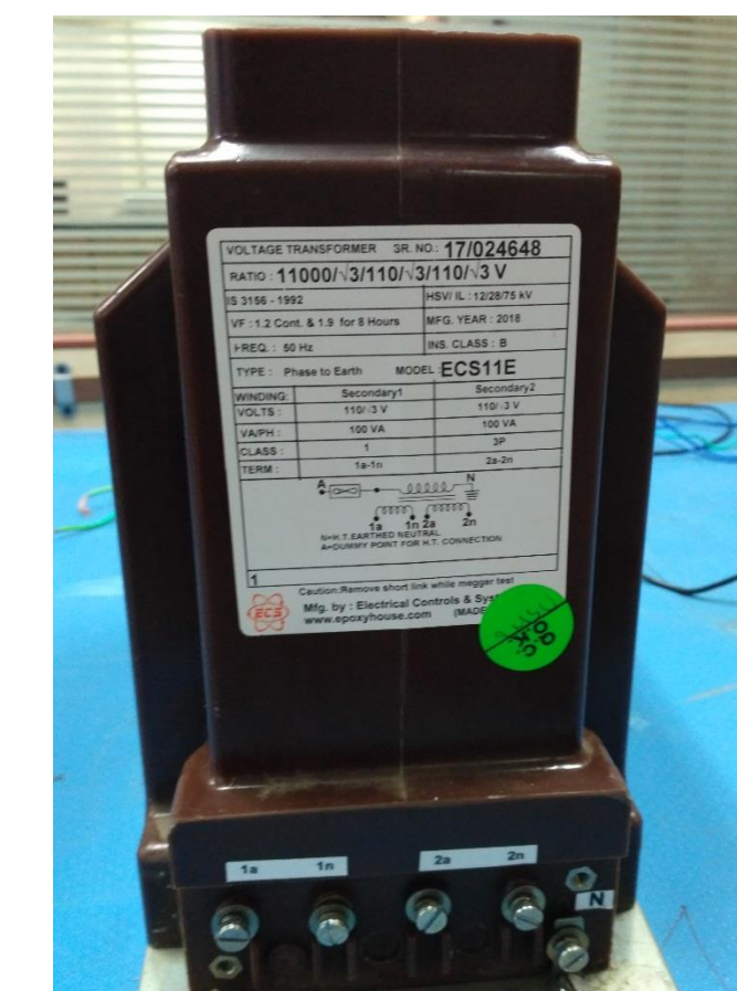
Figure: Epoxy nanocomposite insulation used for fabrication of 11 kV potential transformer
