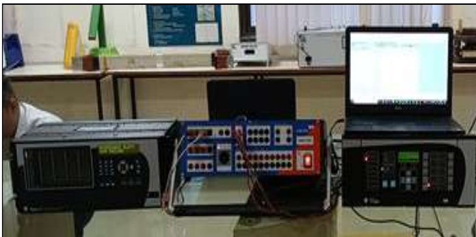
Fig. 5 : Test set up for GOOSE testing as per UCA procedure
