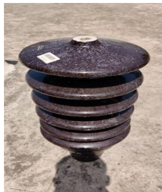
Figure 2: 66 kV Insulator Sample
