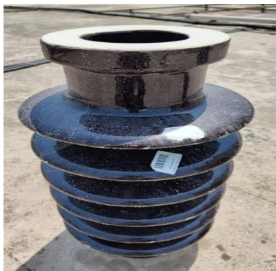
Figure 1: 33 kV Insulator Sample
