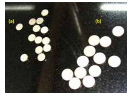
Fig-4: Developed contacts (a) Contact tip with 6 mm diameter (b) contactor with 8 mm diameter
