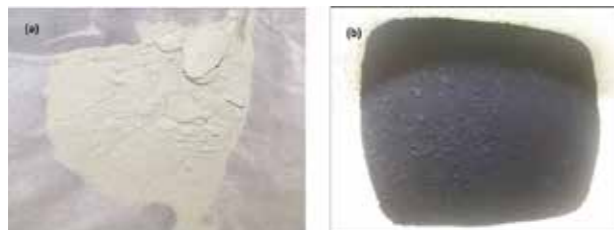
Fig-1: a) Silver powder (b) Functionalized CNT
